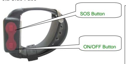
NOTE:As for ON/OFF Button,keep pressing 3 seconds is ON/OFF the tracker;while keep pressing 1 second is switch to displaying Latitude&Longitude.it displays Time,Date,Day and Battery in 30 seconds later automatically.
