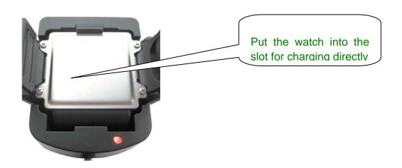
Do charge the battery to capacity in 8 -12 hours for the first use. Please use the battery and charger provided by the manufacturer. This unit adopts built-in Li-ion battery, and full battery will support around 48 hours use on end. After first use, the battery can be charged fully in 3-5hours.
