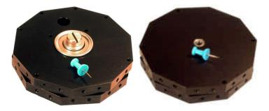
There are a variety of ways to mount devices to the Snap360 turntable. Around the edge of each plate are a series of #6-32 threaded holes. On the face of the plates are four more #6-32 holes. The bottom center of the turntable has a ½-20 threaded hole, which can be used for mounting the entire Snap360 to a tripod, or other standard photographic mount.
