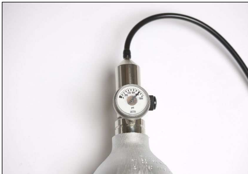
Figure 23 - Flow regulator fitted to calibration bottle
