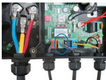
Step 5: Connect "Alarm" Terminal Wires
