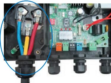
Step 2: Connect "PWR" Terminal Wires
