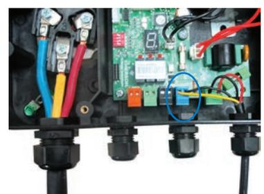
Step 4: Connect "CCC" Terminal Wires
