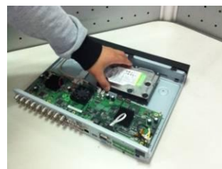
③ Place the HDD in accordance with the four holes in the bottom.
