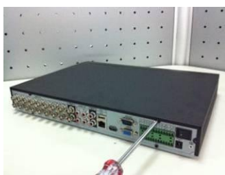
⑧ Secure the screws in the rear panel and the side panel.
