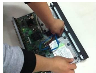
⑥ Connect the HDD cable and power cable.
