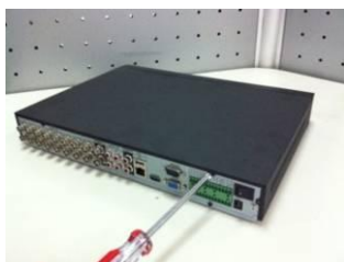
① Loosen the screws of the upper cover and side panel.
