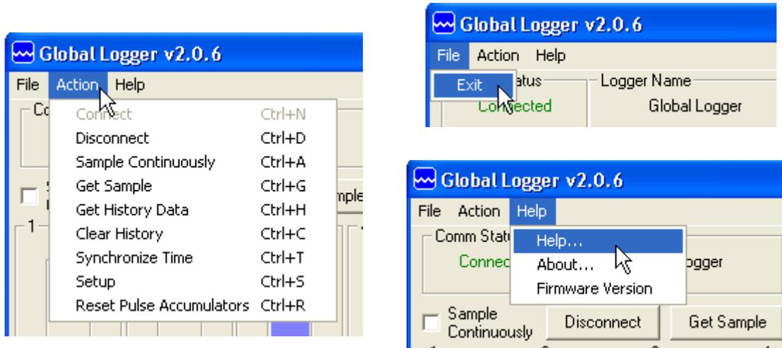
**COM Status:** This reads “Connected” in green or “Not Connected” in red, depending on the current connection status.
