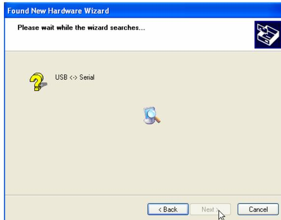
5) The first half of the installation is complete. The Hardware Wizard must make two passes.
