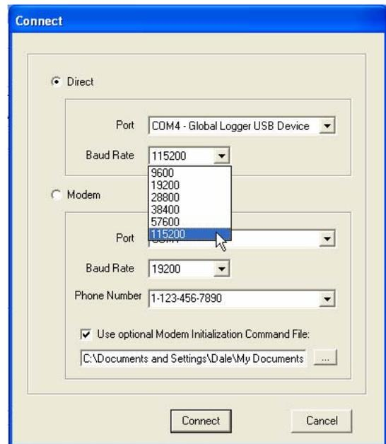
To connect to the logger, click the “Direct” option and from the “Port” menu, select the USB serial port at the COM port the driver was assigned, which is automatically shown in the list as “Global Logger USB Device”.
