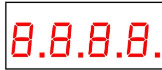
When turned on the ST314A performs a display test by briefly illuminating all of the display digits and all of the front panel lamps.
