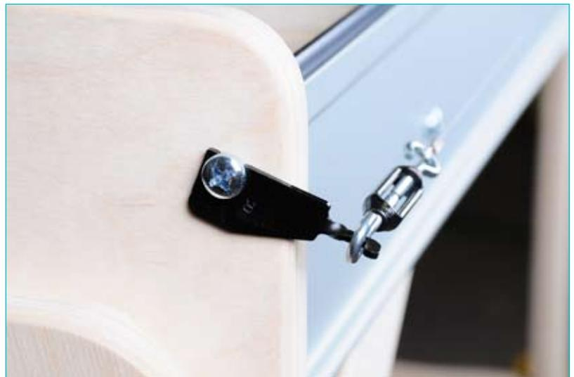
Attach one end of the drive wire to the X-axis bracket as shown in the top photo. Wrap the wire around the drive wheel twice and ensure that you start at the TOP of the wheel as shown in the photo to the left. Attach the other end of the wire to the tensioner as shown in the photo above. Finally attach the other end of the tensioner to the X-axis bracket as shown above. Use the tensioning template in the back of the User Manual to set the proper tension in the wire.
