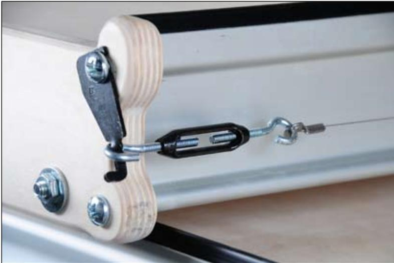
The front attachment looks like the picture to the left. The drive wire is shown installed and the tensioner has been adjusted to the correct tension using the tensioning template found at the back of your QBOT manual.
