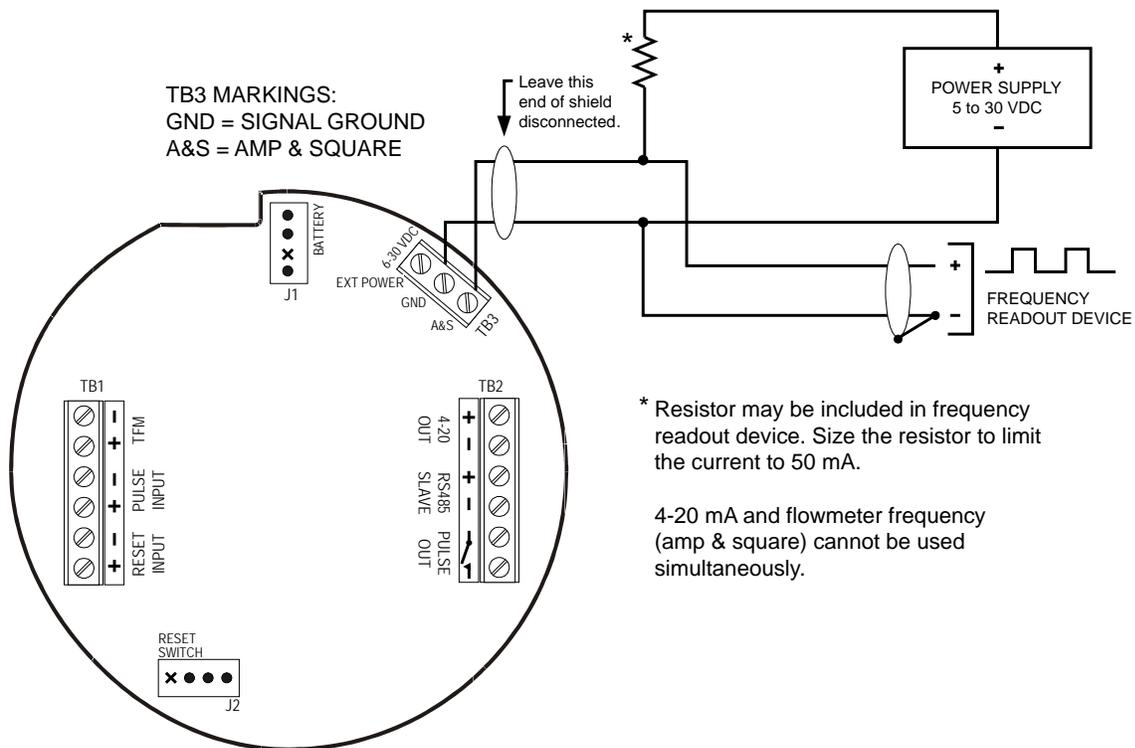
Figure 2.15—Flowmeter frequency (amp & square) output wiring
