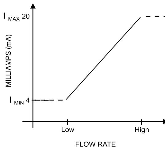
Figure 3.2—4-20 mA output configuration
