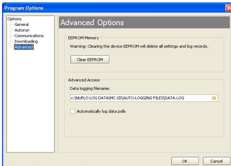
Figure 6.7—EEPROM clearing and automatic data log option
