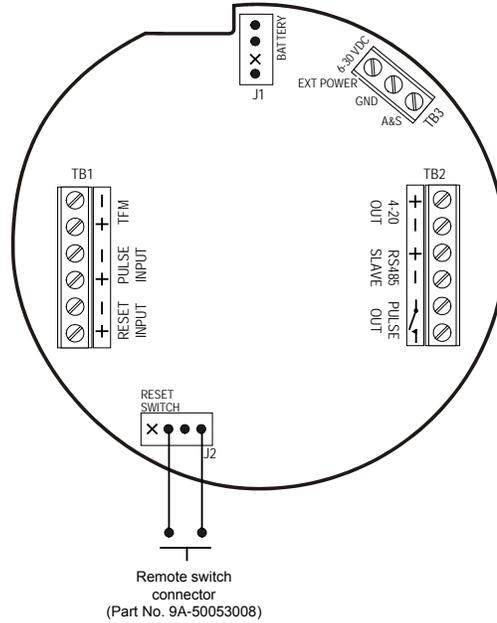
Figure A.2—Explosion-proof switch wiring
