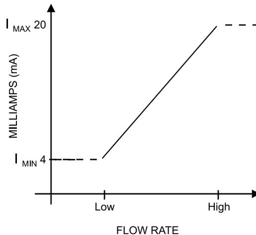
Figure 4.29—4-20 mA output configuration
