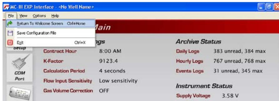
Figure 4.37—File dropdown menu allows user to return to the Welcome screen
