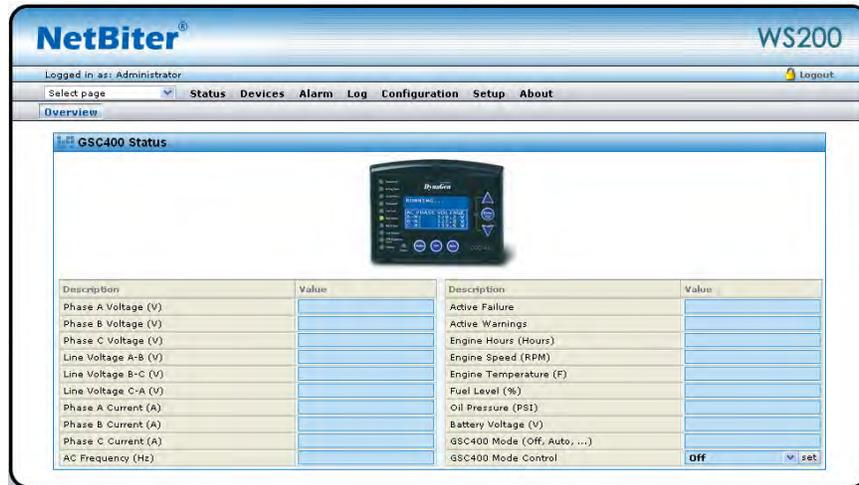
The screenshot shows the NetBiter WS200 web interface. The top navigation bar includes 'Status', 'Devices', 'Alarm', 'Log', 'Configuration', 'Setup', and 'About'. The 'Overview' section is active, displaying the 'GSC400 Status' page. This page features a central image of the GSC400 device and a table with the following data:
