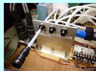
Photo 9 Gas inlets A tube diameter conversion adaptor is attached to the Air terminal on the left.
