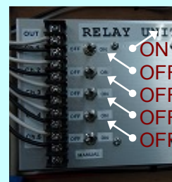
Photo 4 Settings for relay unit. (Only OUT channel 1 is on.)
