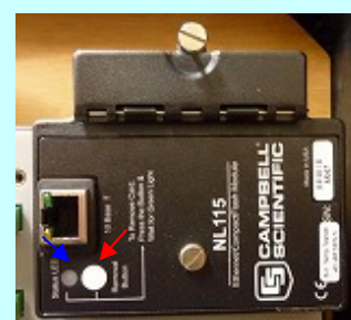
Photo 11 Removal button (→) and status LED (→)
