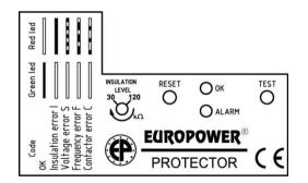
Fig. 1.3 Schematic representation of the front panel
