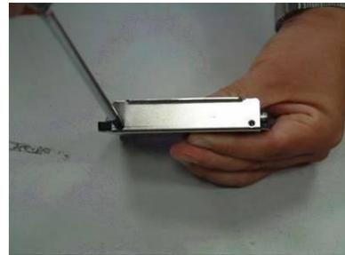
Step 5: Plug HDD cable. Pay close attention to SATA power cable and SATA cable at the right position.
