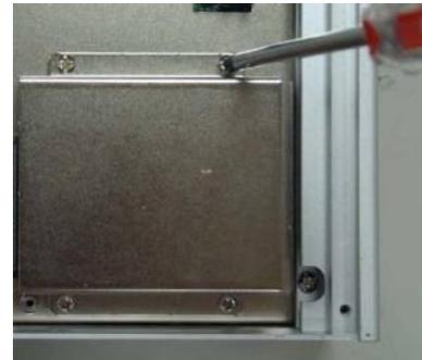
Step 7: Put bottom cover back in place and screws it.
