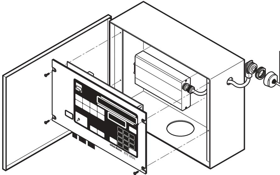
**Figure 4: Permanent Mount Pro Max Receiver**
