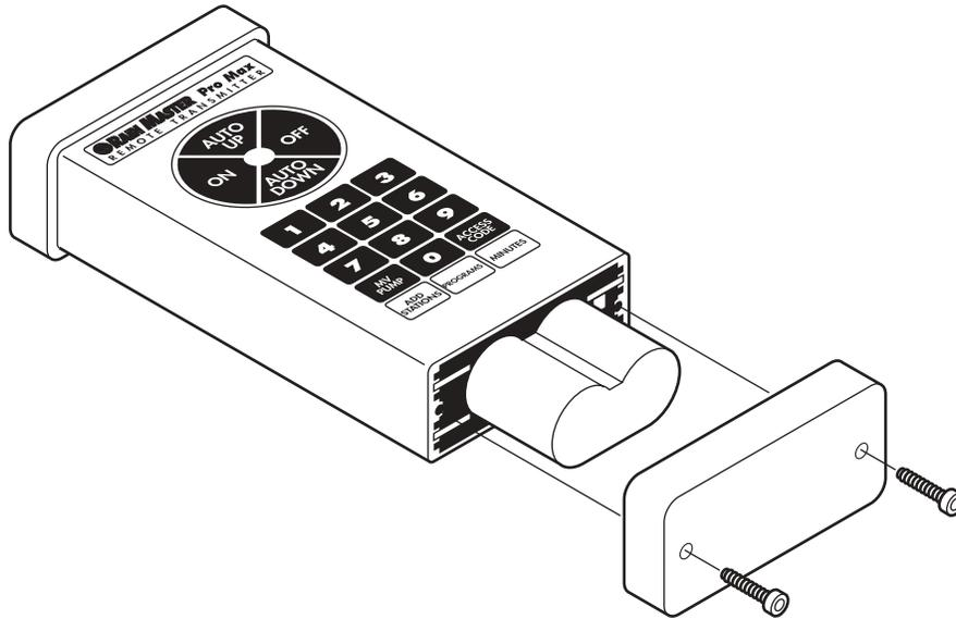
**Figure 11: Battery Replacement**
