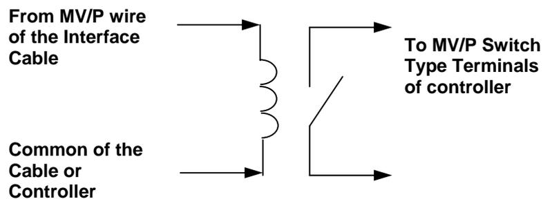
**Figure 7: Relay (such as Rain Master RLY1)**
