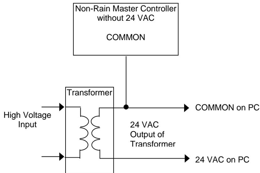
**Figure 9: Non-Rain Master Controller 24 Volts AC**
