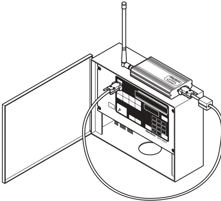
**Figure 3: Pro Max Receiver to Rain Master Controller**
