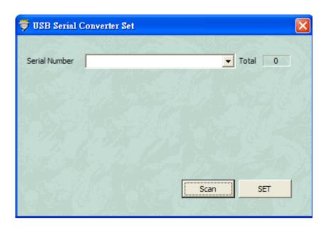
Click **Scan** button to locate all the RS-422/RS-485 serial server on line, selected the desired serial server on list
