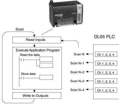
Analog Module Even though the channel updates to the CPU are synchronous with the CPU scan, the module asynchronously monitors the analog transmitter signals and converts each signal into a 12-bit binary representation. This enables the module to continuously provide accurate measurements without slowing down the discrete control logic in the RLL program.
