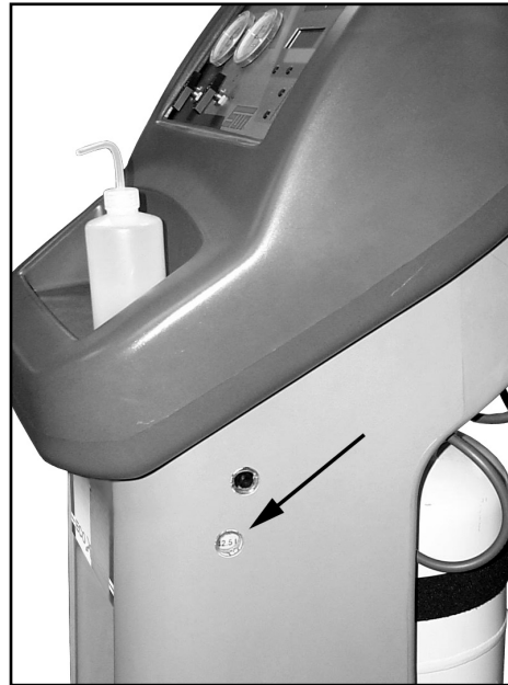
Figure 3-5: Oil Level Sight Glass
