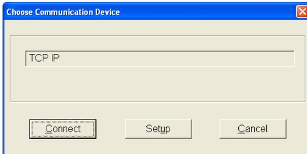
Using the Setup button the IP address and the listening port of the server can be set. These values are remembered in new sessions after exiting
