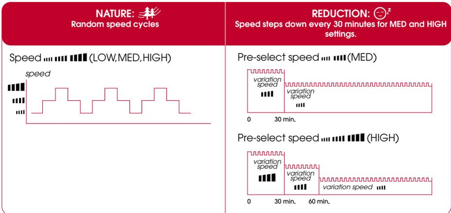
**NOTE:** When the NATURE mode setting is selected, the tower fan is programmed to self regulate through the various fan speeds. The NATURE mode is independent from the fan speed settings while the LED screen will still display the last selected fan speed setting.
