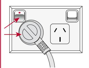
Plug the cord into a 230V or 240V power point and switch on.
