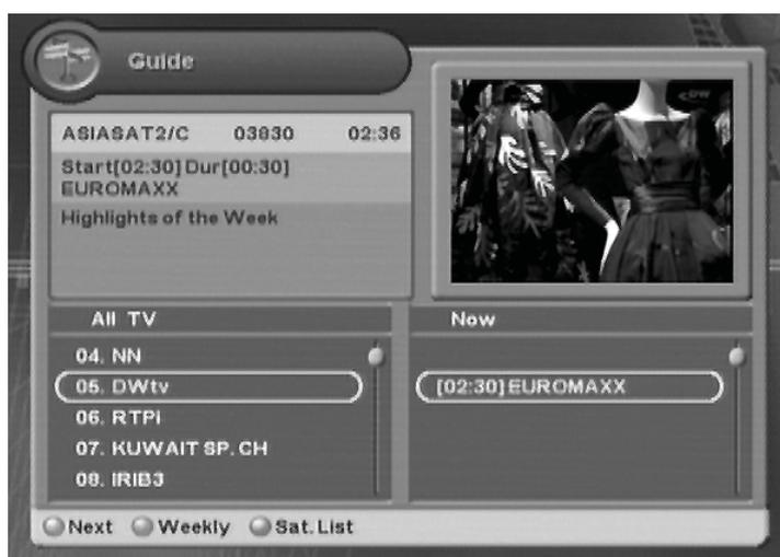
Move to other desired channel using the “▲▼” button. If there are multiple channels, use the “PAGE▲▼” button to move to channels by page.
