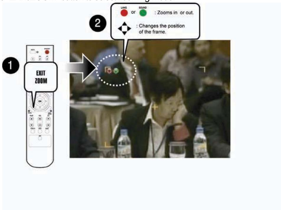
3. Press the “Red” button to zoom in the screen or the “Green” button to zoom out the screen. Or press the “◀▶▲▼” button to change the position of the frame.
