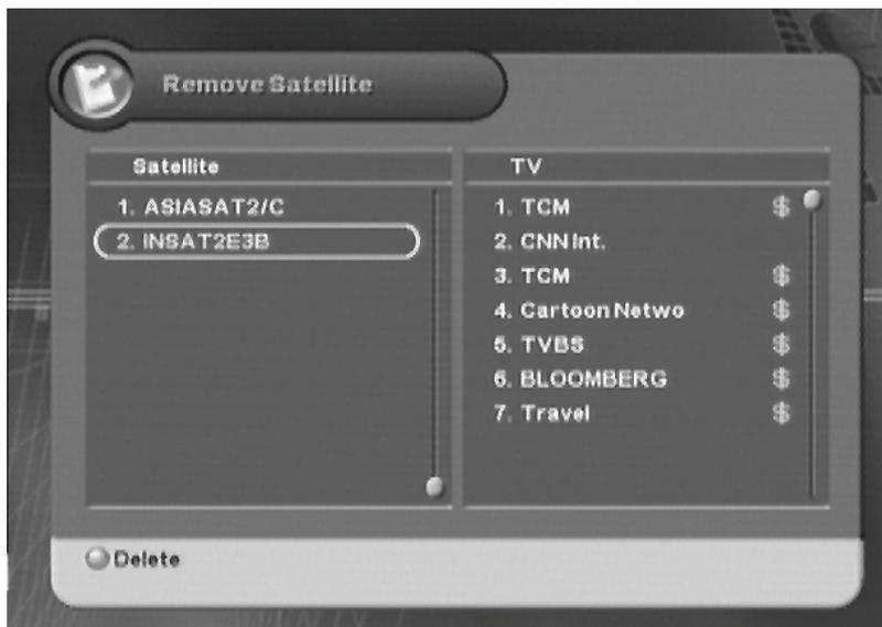
3. Press the “Red” button to delete the channel(s) for the satellite.
