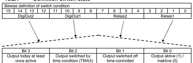
(The definition of the switch state with bit 0, bit 1, bit 2, bit 3 is possible in each case for both relays and both digital outputs)
