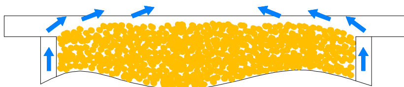
Figure no. 18. Situation of pellets in relation to retort burner when boiler operates
