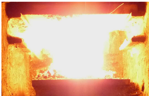
Figure no. 15. Retort burner's operation during combustion of coal, Ling 15 – 50kW.
