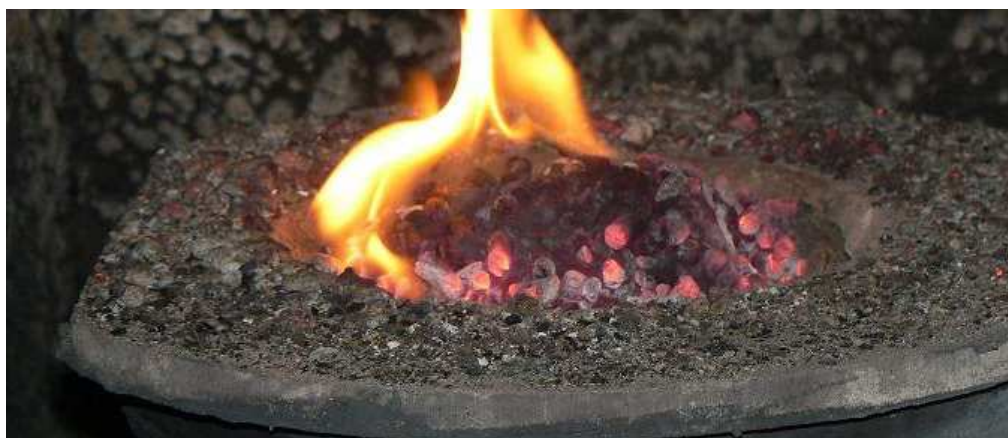
Figure no. 19. Situation of pellets in relation to retort burner when boiler operates Ling 15–50kW.
