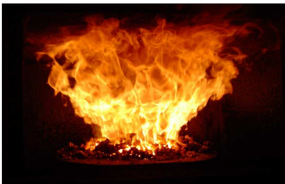
Figure no. 16. Retort burner's work during combustion of coal, Ling 75kW.
