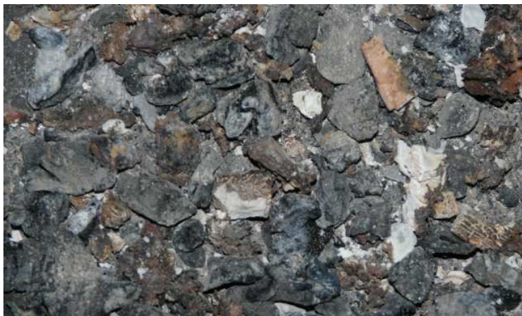
Figure no. 17. Coal sintering (caking) – incorrect regulation of burner in relation to fuel quality.
