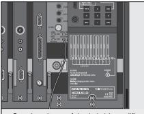
Supply voltage of the hybrid amplifier (+24 V---- via the screened lead)
