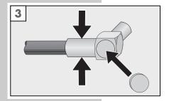
3 Use appropriate crimp pliers to firmly press together the metal shoe (arrow) of the right-angle plug (see Fig. 3). Press the enclosed cover into the opening of the right-angle plug.
