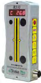
The R310 essentially measures the distance between the work surface and the laser beam. The T330 laser provides a near to 360° laser plane. Sensor “reachability” of around 80m The sensor has a keypad giving complete access to all features without the need for a PC. Real-time measurement values over the LED Display If required, Bluetooth communication with a PC is possible using a combined BT/ Battery pack
