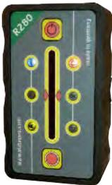
The R280 essentially measures the distance between the work surface and the laser beam. The T330 laser provides a near to 360° laser plane with a Sensor “reachability” of around 80m. Bluetooth communication with the PC and a changeable Li-Ion rechargeable cell giving 8 Hrs measurement time.
