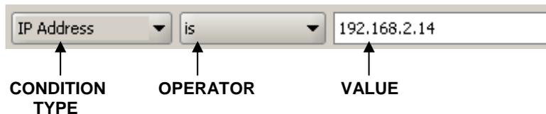
This toolbar lets you create a filter condition by specifying the condition type, operator and value from the corresponding drop-down lists/input lines. Once the condition is configured, you can add it to the filter by clicking the **Add** button in the right section of the dialog box. Added conditions appear in the Conditions panel below the New condition toolbar.
