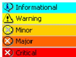
The [severity level](#) of an active alarm can be **Informational**, **Warning**, **Minor**, **Major**, or **Critical**. When an alarm is cleared, its [state](#) changes from **active** to **cleared**, however, the severity level of a cleared alarm does not change. By default, cleared alarms have green background color.
