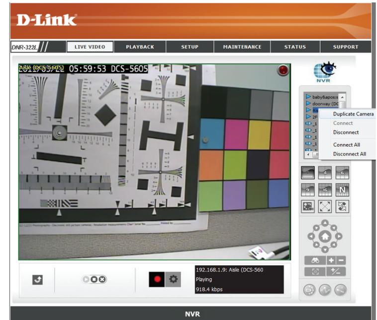
**Duplicate Camera:** Select the duplicate camera function to create multiple views. The duplicated camera will be shown with a green indicator. Combine this function with digital PTZ so users are able to enlarge different spots and view them in different channels. This whole view can be recorded.
