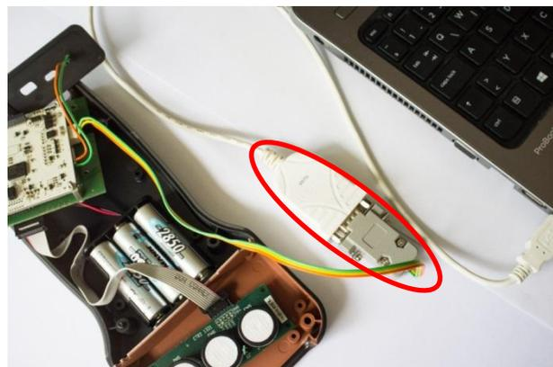
**Figure 22: VESNA SNC board connected to a computer.**
