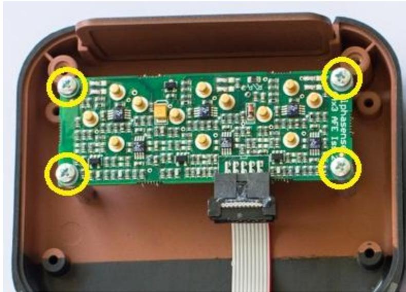
Figure 14: Removing Alphasense AFE board.
