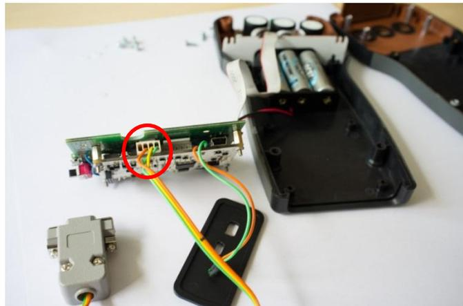
**Figure 21: Serial cable connected to the VESNA SNC board.**
