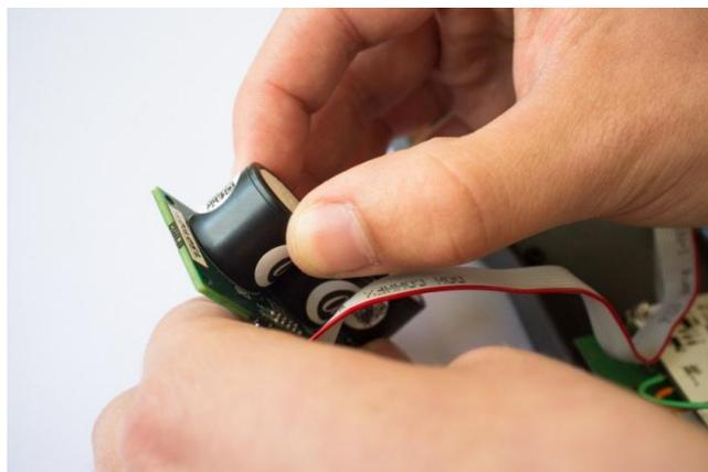
Figure 15: Grab the AFE board and the sensor you want to replace.
