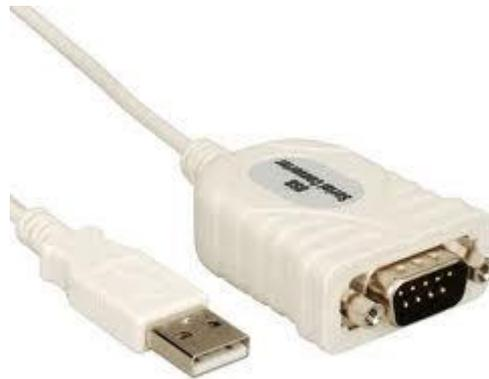
Figure 18: USB to serial connector.
