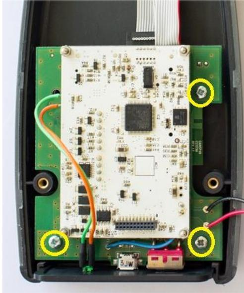
**Figure 20: Removing VESNA SNC and SNE-AQA boards.**
