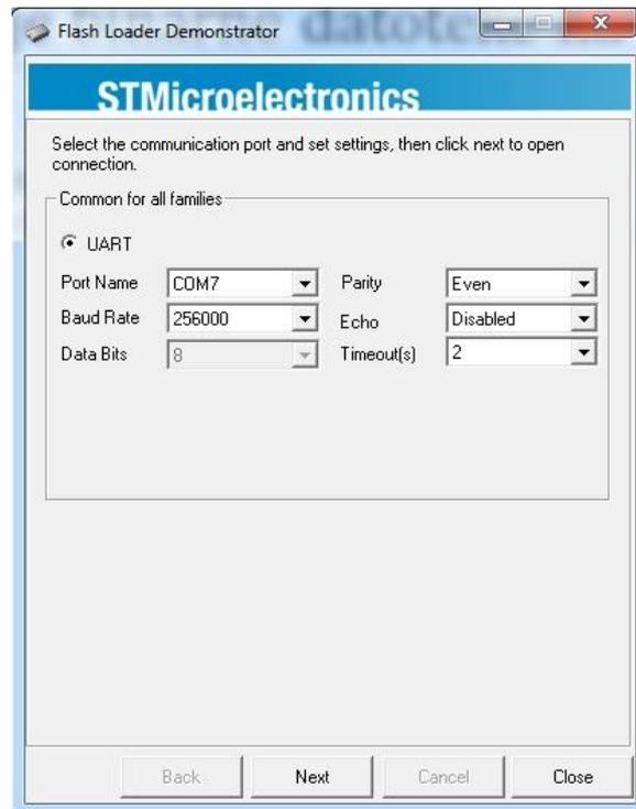
Figure 23: Settings of Flash Loader Demonstrator application.
