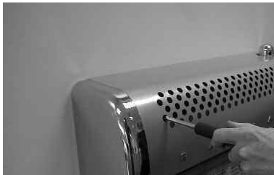
Fig. 10 Removing the Upper Outer Case Fixing Screws
