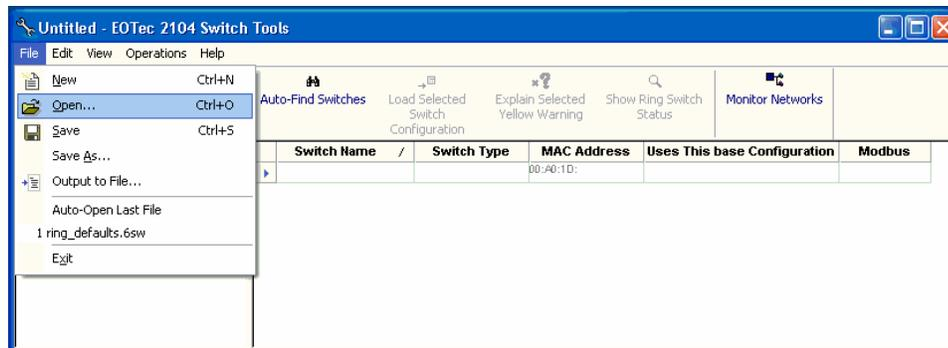
2. Select the file **ring\_defaults.6sw** to highlight it and click **Open**. The default project is loaded into Switch Tools.
