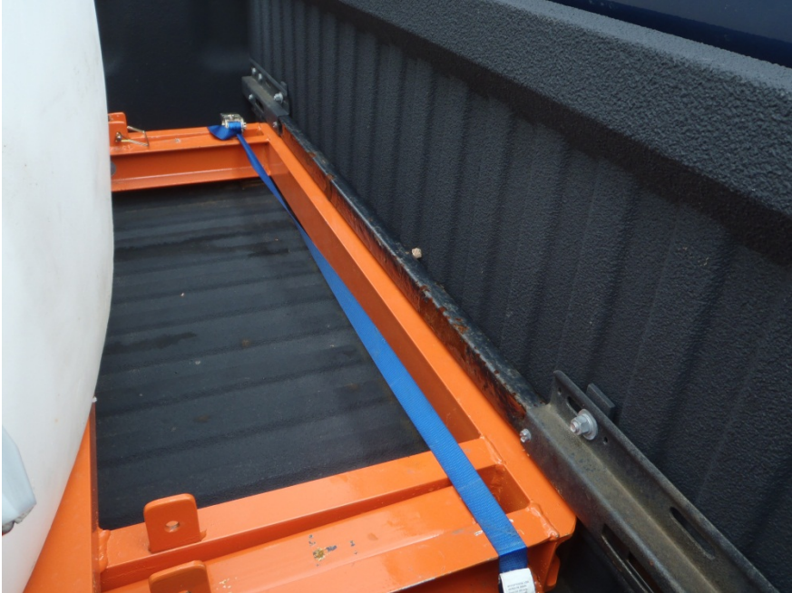
Pic 3- push unit in so frame contacts the bed bulkhead firmly.
