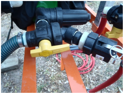
Source valve in fill position.
