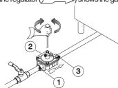
**NOTE!** These models are designed and certified for use with natural or propane gas. For natural gas, the pressure regulator on the header is set to 8" w.c. (20mbar).
