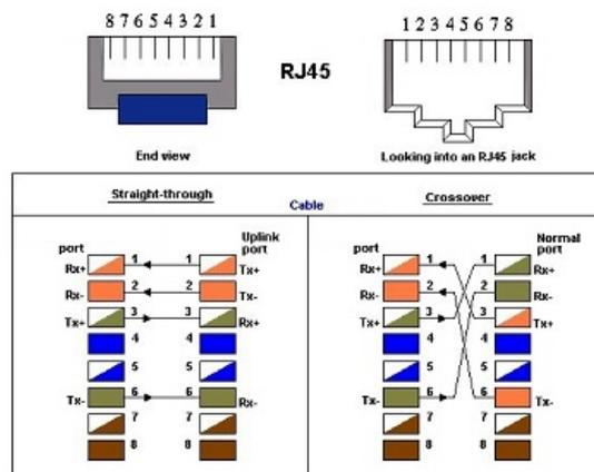
Figure 3.2-4 Ethernet Pin Assignment
