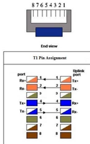
Figure 3.2-5 T1 Pin Assignments
