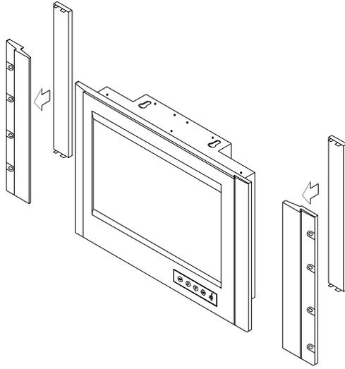
Figure 2.3: Rack Mounting Brackets
