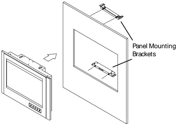
Figure 2.2: Panel Mounting (396 x 296 mm)
