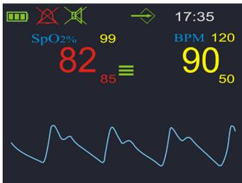
Figure: Visual alarm which was triggered by a violation of the lower SpO2 alarm limit.
