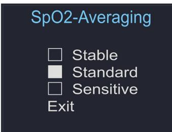
**Stable:** When this setting is selected any strong and sudden variations in data will not immediately affect the reading (data incorporated over time); minor irregularities have little or no effect on the displayed reading.
