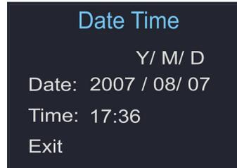
First, select between 12h mode and 24h mode; then set date and time. Settings for date and time are not erased when the batteries are temporarily removed.
