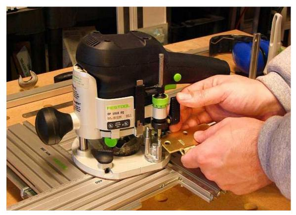
After installing the bit, the next step is to set the router's depth, plunge the router until it comes into contact with the work piece. This is called zeroing the bit. Now, I use the hinge itself between one of the turret stops and the depth rod to set the exact depth.
