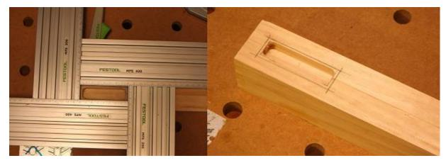
The finished mortise. The angle stops make it a breeze to set the MFS up quickly when you need to rout the same location/size mortises on multiple work pieces. Just imagine the ease of routing traditional M&T joints for table and chair legs or mission style furniture.
