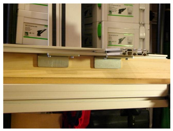
Here the angle stops are mounted on the bottom of the MFS to precisely locate the MFS for an inlay.
