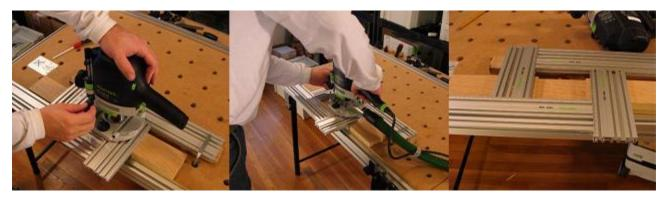
More of the same; set the depth of the bit and rout. I need to be a little careful because I'm routing off each edge, and tear out can happen here. Removing small amounts near the edges will greatly reduce the chance of tear out.
