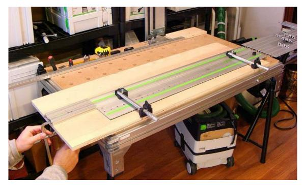
I've struggled to find a good way to use the 42" LR32 rail on stock longer than the rail itself. No problem; install a guide rail connector to join an MFS profile to the rail and clamp the profile to the edge of the stock. Now drill your holes.
