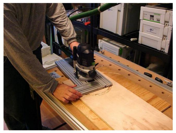
All right, back to the example. I have a 10 mm bit in the router and the insert set to cut a 100 mm outside radius (90 mm inside). My MFT has a piece of scrap on it to protect the top, and the work piece has double-sided tape to hold it down to the scrap. I've dropped the pivot in the pilot hole, set the depth of the bit to 8 mm. Plunge the router and start turning the template on the pivot to rout the circle.
