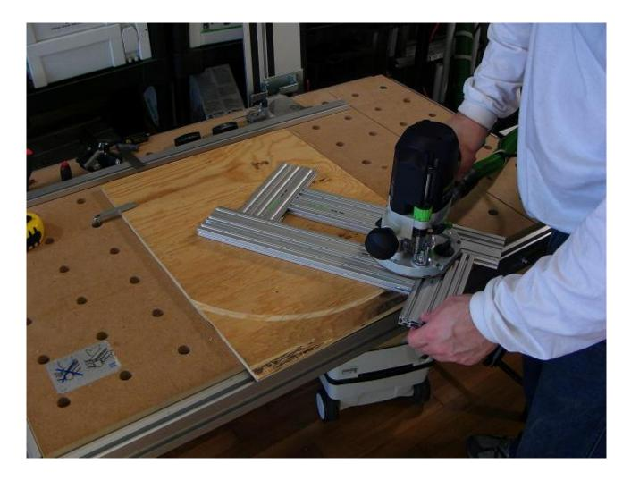
Slip the pivot in the pilot hole, set the insert to the desired radius and tighten it in place, then set the copying ring/router in the insert. The template and router pivot around the stock to cut the circle. You can see from the picture that I'm working out the process on scrap first before committing to the real work piece.
