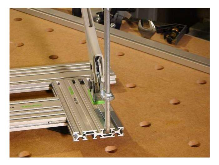
The Festool <u>FSZ 120</u>, <u>FSZ 300</u> and <u>FS-HZ</u> clamps fit in the clamp slots, as do the <u>guide rail</u> <u>connectors</u>. The guide connectors can also be used to join the profiles in length. Also, 1/4" square and hex nuts fit the slots if you want to add a fixture to the profiles or mount them to jig or table with your own (imperial or "inch" style) hardware.
