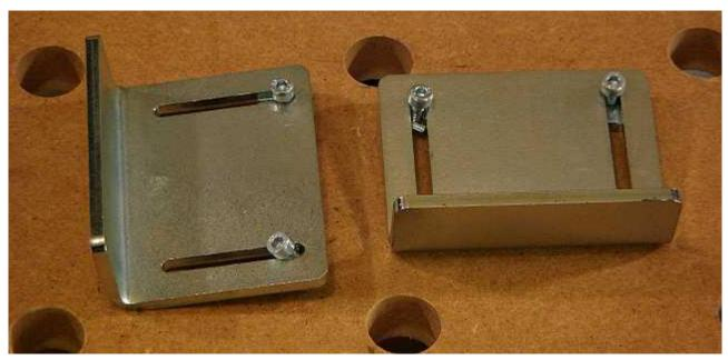
The angle stops mount into the V slots and are used to help position the MFS.
