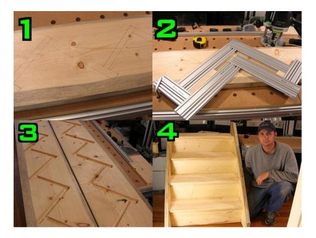
I also routed stringers for a small staircase. This is where having both the MFS 400 and 700 sets really paid off. Two sets allowed me to make the L-shaped template I needed to rout in the treads and risers for this job. You may never need to rout stringers, but it is nice to know you can. More details can be found in my "Projects" page, <u>Small Staircase</u>.
