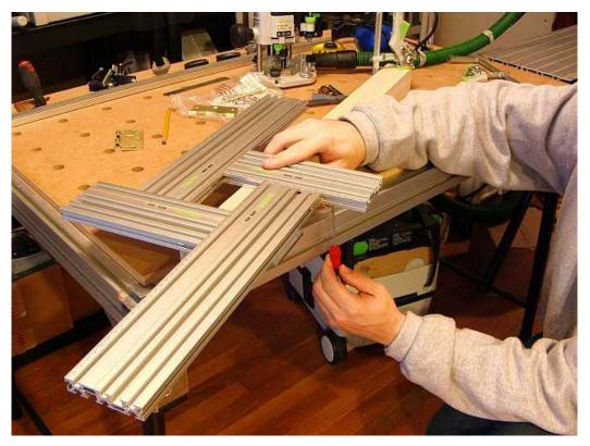
Once the MFS is set to size, I place it on the pencil line then set the angle stops and clamp the work piece/MFS down.
