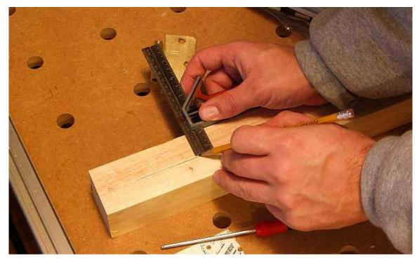
The first step is to mark the setback for the hinge. I'll use this line to index the MFS.
