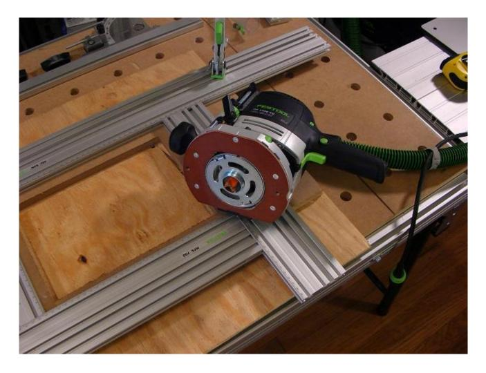
I've switched to my OF1400 router to make the lip for the plate. I've already put an 18 mm bit and a 30 mm copying ring in the router, I set the MFS for the 7 mm offset. The 18 mm bit should fit the radius on the corners of the plate perfectly.
