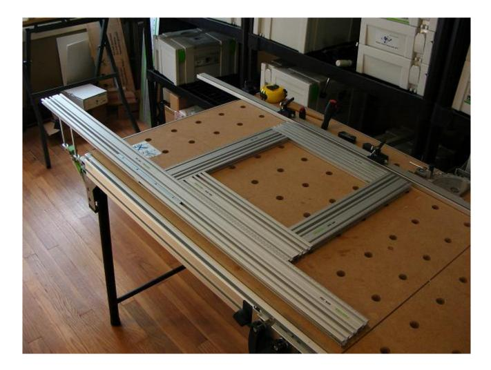
Here is a look at Jerry Work's idea of how to use the MFS as a fence for cutting and routing with the MFT. It consists of profiles to form a square or rectangle and a single long profile as a fence. The scales on the profiles are used to set the distance from the square/rectangle to the guide rail's rubber splinter guard.
