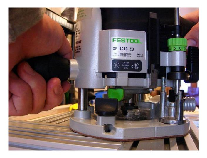
For circle cutting the MFS 400 has a maximum diameter of around 32" and the MFS 700 around 55". For template routing the 400 set's maximum size is about 4 11/16" x 12 9/16", the 700 set 12 9/16" x 24 7/16". Combining sets and/or the longer profiles greatly increases these sizes (and the usefulness of the MFS system as a whole).
