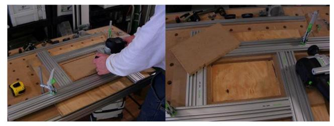
The bit is set to cut all of the way through the MDF, so I placed a scrap under the work piece to protect my MFT's top. I'll guide the router slowly around the template.
