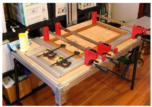
Clamps can be added almost any place needed to square the frame.
