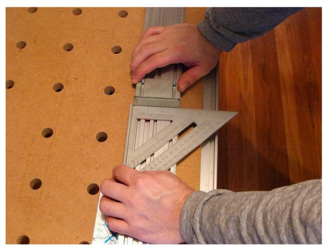
Using an MFS profile as a story stick is an easy way to accurately place Festool's guide rails. I use one of the angle stops with a profile to set razor blades to act as stops for the rail, <u>John Lucas' idea</u>. Install the angle stop in the profile, with the scale up. Using the scale I set the square on the measurement I want. Then butt the stop up to the square and tighten the bolts.
