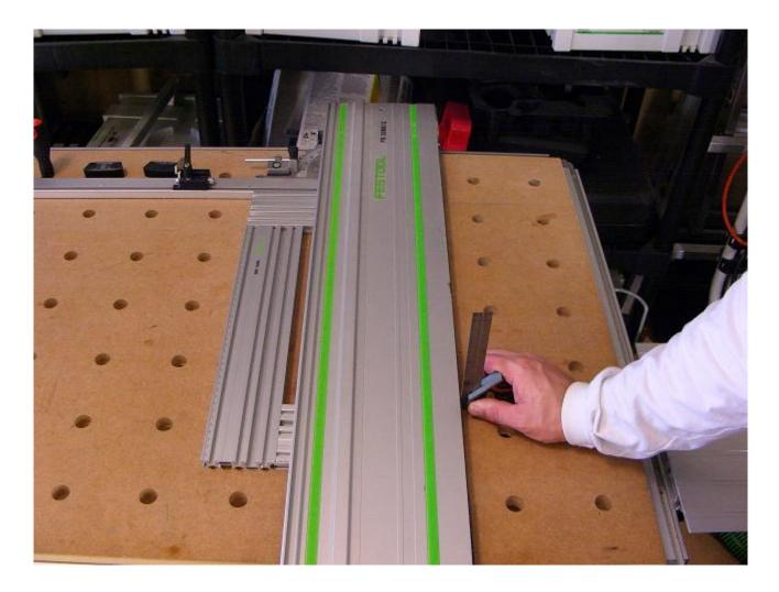
Step one in the setup is to assemble the profiles with the scales on the outside and checking to make sure the setup is square. Now, I slide it under the guide rail and set the edge to be even with the rubber splinter guard on the rail.
