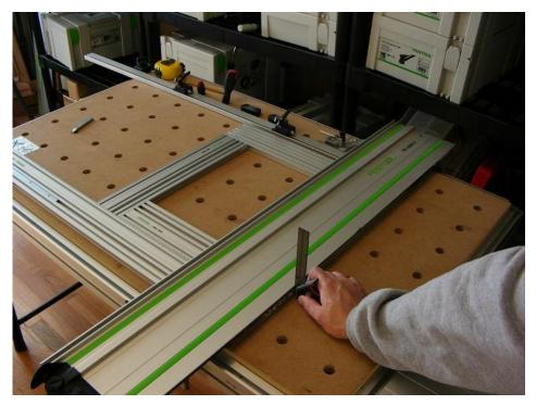
The next step in the process is to set the square to the guide rail's edge, like I did with the setup for narrow rips.
