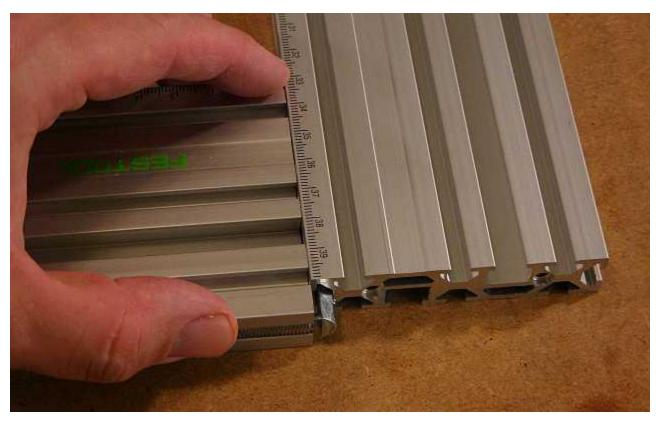
The V nut on the male end of the profile fits into the V slot in the edge of another profile. The male's indexing pins also fit into the edge V slots to ensure perfect alignment.
