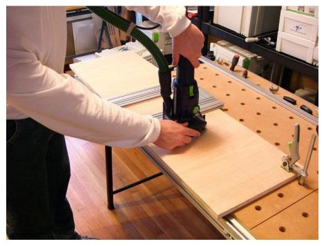
With the base of the Domino against the MFS profile, I can cut all of the mortises in a perfectly straight line, at a right angle to edge of the work piece. Using the center line on the Domino's base and the scale on the MFS, the mortises can be cut quickly and accurately. I would normally use the backside of the guide rail on the MFT for this, but when I'm on a jobsite without my MFT this really comes in handy.
