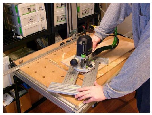
Now I want the center cut out, leaving the lip. I've changed bits, a 6 mm spiral bit now in the router. I'll move the insert to cut a 90 mm outside radius for the 6 mm bit. The depth is set to cut all the way through the stock.
