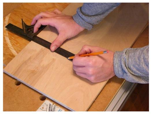
Step one is to lay out for the pivot point, then drill the pilot hole.
