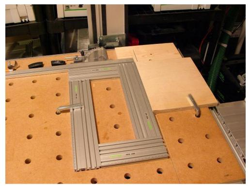
The MFS has to be clamped in place to prevent it from moving during the cut, I also clamp the stock to be extra safe.
