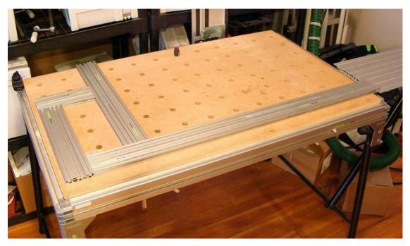
The MFS profiles offer a lot of options for different configurations. I use one shown here most often for clamping face frames. Once the profiles are clamped to the MFT they provide a sturdy squaring fixture.
