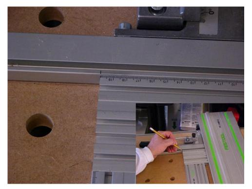
One of the things that makes this technique so fast and easy is using the scale on the MFS to set the width of the rip. With the MFS lined up with the rail make a pencil mark at the profile's zero point (end of the profile). With this mark I'll be able to use the scale, in reverse, to set the width of the rip.
