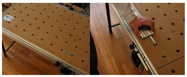
To hold the two profiles that will be the fence, two clamps are placed in from the bottom the MFT. Then the profiles slide onto the clamps. The clamps are not tightened yet. That gives me what you see in the first picture on this page.
