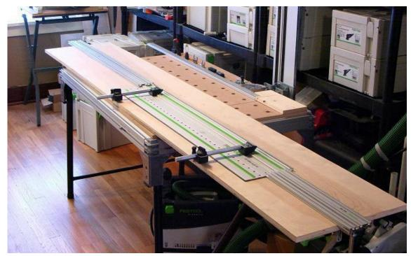
Stock eight feet long posed an even bigger challenge. Using the same technique and the circlecutting pivots to re-index the rail, you can drill holes in a full sheet of plywood.
