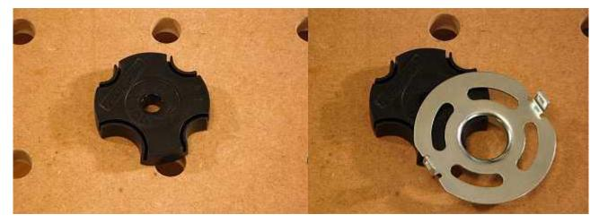
This is the anti-tilting insert. It is used to prevent the router from tipping or tilting during routing operations. If the router is tilted the work piece can be ruined. Copying rings fit into the anti-tilting insert, this allows it to travel with the router. The insert can fit 24, 27, 30 and 40 mm copying rings.
