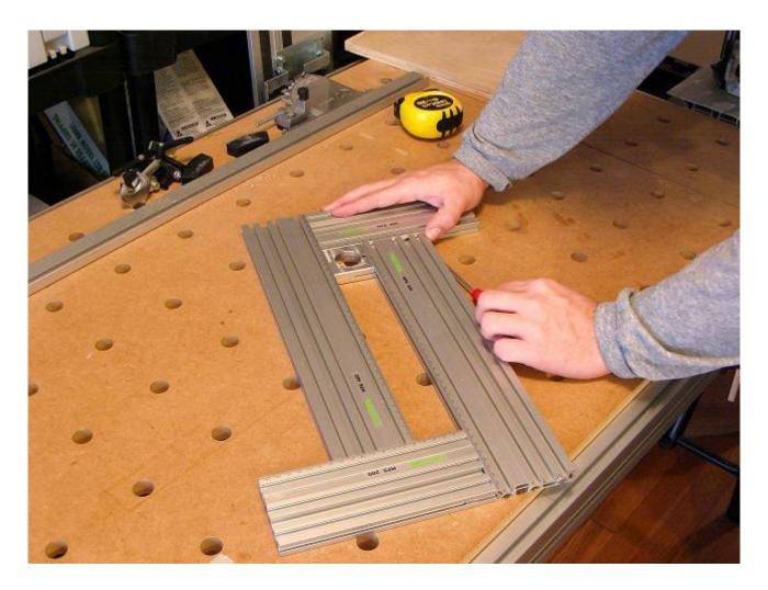
I'll start with a quick overview of the process for circle cutting before I go into detail. The circle-cutting insert fits into the interior V grooves of the profiles, the template is closed on and capturing the insert (see photo above). A 30 mm copying ring fits into the insert, so the next thing to do is install the ring in the router.
