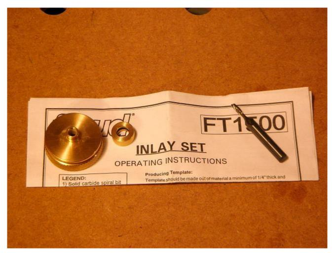
Taking offset routing one step farther, we'll take a look at making the male portion and female recess for inlays with the MFS. Keeping the MFS the same size and changing the copying rings/bits allows inlays to be cut quickly and accurately.
