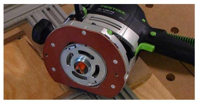
Let's now look at using copying rings or guide bushings with the MFS. The advantage of using copying rings is twofold: they are always in place while routing, greatly reducing the chance of cutting into the profile; and they work with most bits used for template routing, regardless of the bit's cutting length. Unlike bearing-guided bits where the cutter's length is so important. Of course you do have to account for the offset between the bit and the copying ring when setting the MFS to size.
