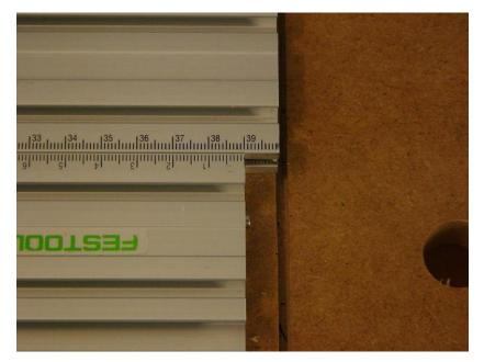
This is a close up of the offset of the scales. The 39 cm mark on the zero point of the fence's scale. Now to set the distance of the square from the guide rail I use the scale on the fence profile.
