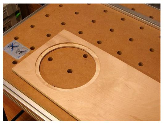
I'm going to start by showing the finished piece for this example so you can see what I am setting up to rout, a cutout with a lip or rebate.
