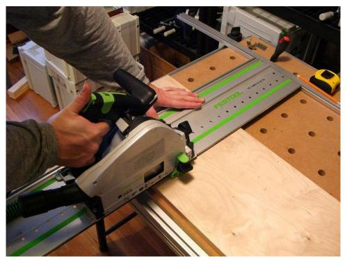
Be sure to remove the razor blades before you make the cut. Use this technique any time you need to make multiple cuts the same size. It works just as well with short or long rails.
