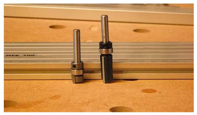
The picture above shows the potential dangers of using a pattern bit with the MFS. I'm not suggesting pattern bits can't be used, but, care must be taken when selecting the right bit. Bearing size, cutting length and diameter should all factor into the decision. When used in the right circumstances they can be a real asset.
