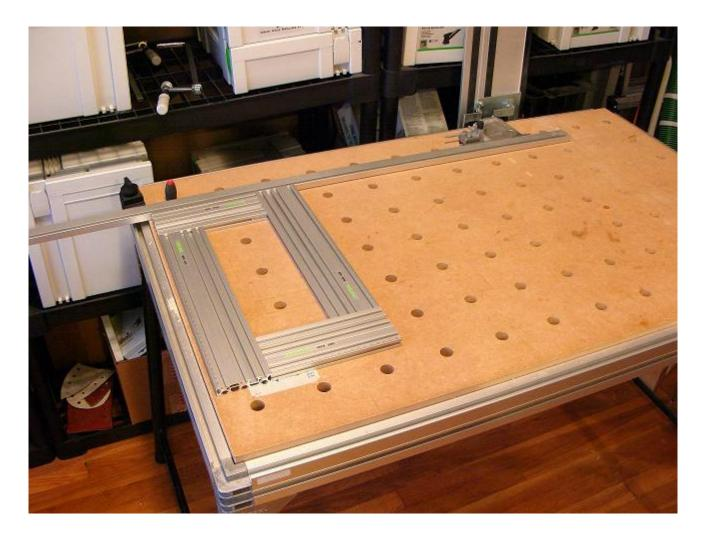
Both the MFS 400 and 700 sets were used in the configuration shown above. A much simpler version for smaller projects can be made from the MFS 400 set. The profiles are clamped against the MFT fence, making a perfect right angle clamping jig, as seen in this picture.
