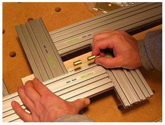
With the small pattern bit I use to rout my hinges I can set the MFS to the exact length of the hinge. The width is set wide enough so I can test fit the hinge without removing the MFS.
