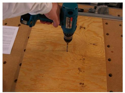
We need a hole for the pivot to go into. An 8 mm or 5/16" drill bit will do the job.
