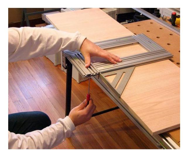
I've used the MFS to index my Domino to cut mortises in the middle of panels. I set the angle stops to square the profiles to the edge of the work piece so the zero point is right on the edge. This will let me use the scale on the profiles to index the Domino.
