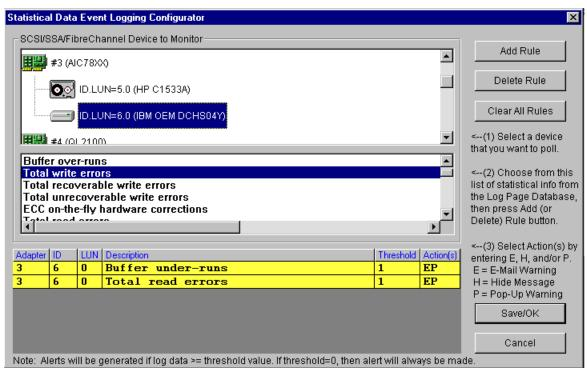
When you pull up this screen, it will guide you through configuring alerts for specific devices. First click on the top window to select a controller, then device to report on.
