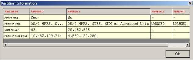
Partitions are an important issue when it comes to hard drives and operating systems. They allow a person to break down a single hard drive into multiple areas that look like smaller hard drives. This is accomplished by reserving the very first sector on the hard drive for a Partition Table. Different Partitions can have, for example, different operating systems on each, so that, by way of an intelligent boot-loader (in the MBR) you can select which operating system to run.
