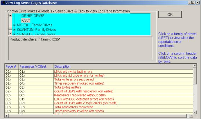
Log sense information is used to track running totals. Typical fields include numbers of read/write errors, cumulative bytes written, temperature, and hours powered-on.
