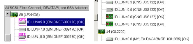
In the image above, The disks at SCSI ID 5 and SCSI ID 8 are installed in a SES enclosure, attached to fibre channel controller #9. The SAF-TE processors are addressed as ID 0, LUN#6 and LUN #7. Note also that SES enclosures specify one or more disk drives in the enclosure as a gateway to communicate with the SES processor. In the case of SAF-TE enclosures, dedicated LUNs or SCSI ID's are utilized to communicate with the enclosure.
