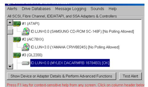
This box shows a tree with all devices and controllers. Click on a device or adapter, then press the <u>Show Disk or Adapter Details & Perform Advanced Functions</u> button to view or modify it's characteristics.
