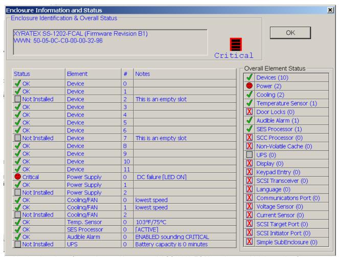
In this situation, the software shows a Xyratex model SS-1202-FCAL enclosure which is running firmware release B1 in the SES electronics. The world wide name for it is 50-05-0C-C0-00-00-32-96. (All fibre channel devices have unique world- wide-names, which are used for identification purposes).
