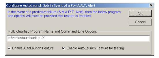
If you click the Enable Auto launch Feature for testing, then this job will begin when you press the Test button on the main screen which will generate a false S.M.A.R.T. error. Use this feature to verify that everything is set up.
