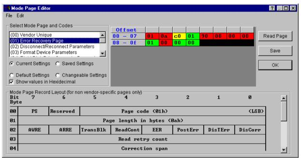
By viewing and modifying mode pages, the user can define a target's operational parameters, such as how a device sets up caching, or how it deals with error recovery or power conditions.
