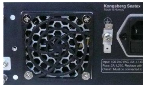
Filter cover removed
