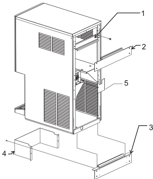
**Installation:** Check building wall for the strength required to support a machine of this weight and size. Note that if at least 6" of space is not left above the machine, cleaning and most service of the machine will require removal of the machine from the wall mounts. All utilities are to be routed thru the base. The back panel is not used when the machine is hung from the wall.
