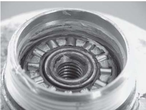
Greased Thrust Half of Bearing
