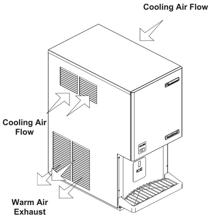
The machine will require electrical power, water and a drain. Follow all local codes. Rough in the utilities before placing the machine into position (see For The Electrician and For The Plumber).
