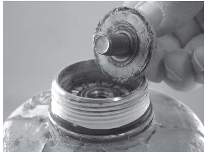
Thrust Washer and Bearing
