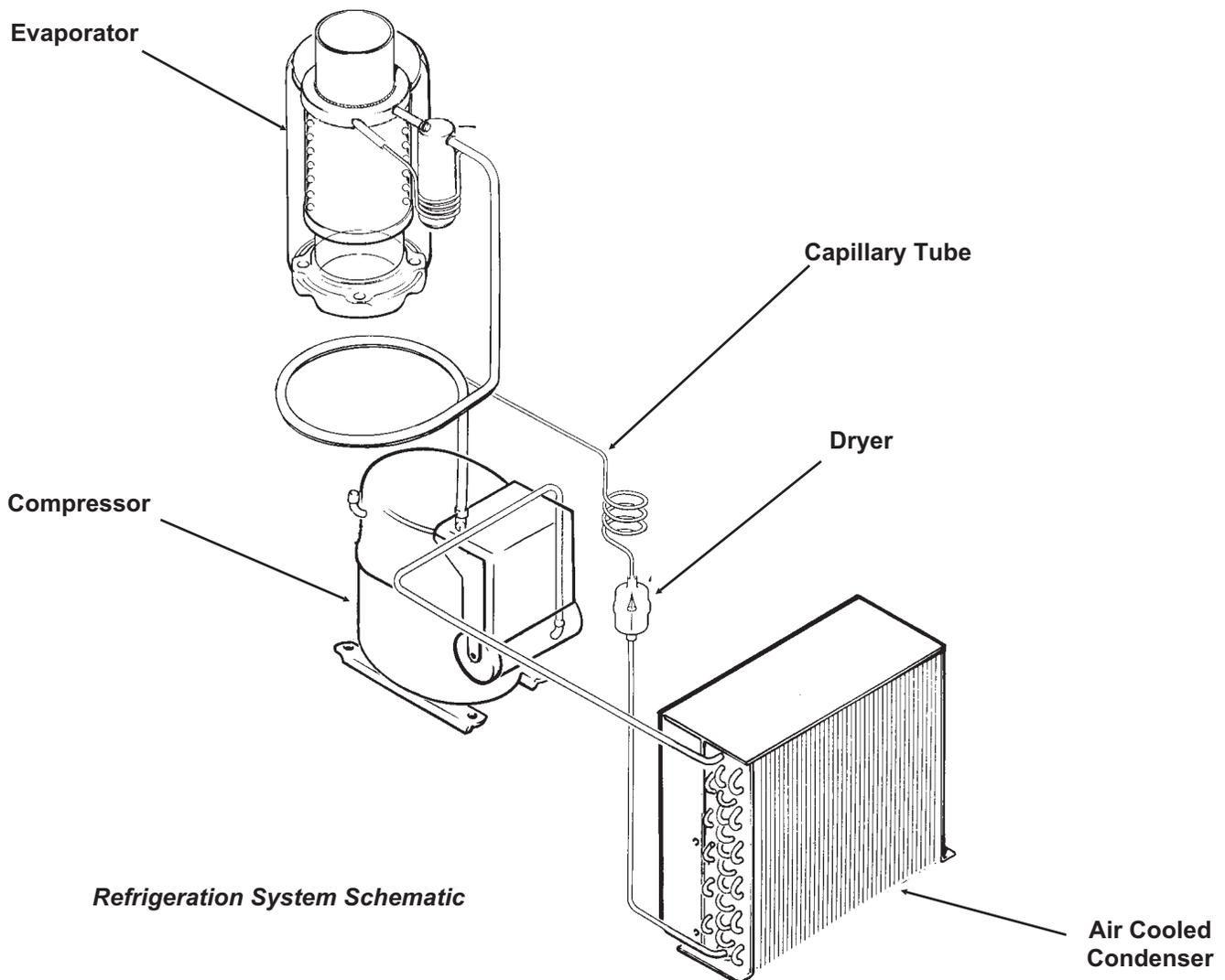
*Refrigeration System Schematic*
