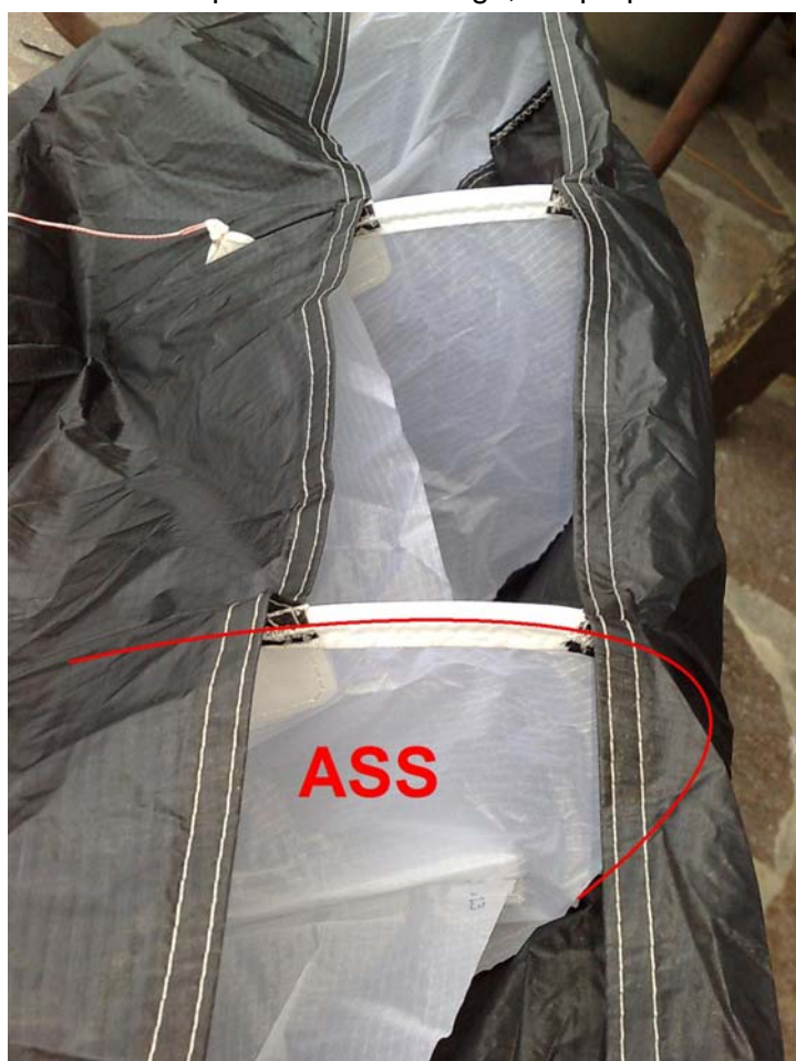
The ASS Leading Edge reinforcement system significantly reduces canopy weight and guarantees perfect inflation even after many years of frequent imperfect canopy folding
