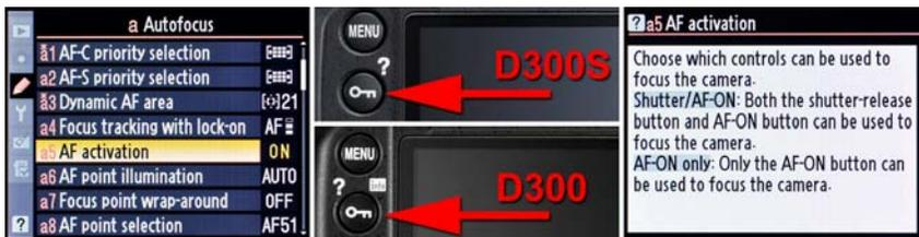
FIG 14 – Help button for Custom Setting a5 > AF activation
