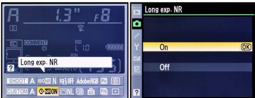
FIG 9 – Information display edit screen – Long exposure noise reduction
