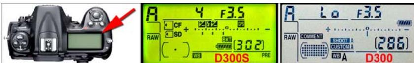
FIG 13 – Control panel LCD screen – D300S (green) and D300 (silver)
