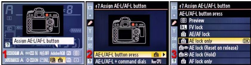
FIG 11A – Information display edit screen – AE-L/AF-L button press
