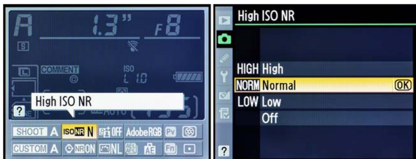
FIG 4 – Information display edit screen – High ISO noise reduction
