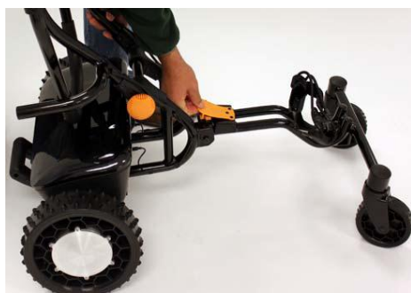
4. Push tab down to lock wheels in place
