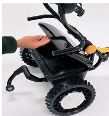
7. Lift battery cover to open
