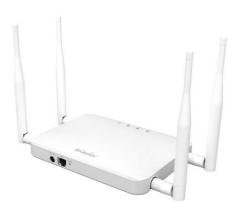
**ECB600** is a wireless-11n 600Mbps (300Mbps + 300Mbps) Dual Band concurrent Access Point/ Client Bridge. It allows simultaneous operation of 2.4GHz and 5GHz wireless network. With media-optimized performance, you can enjoy internet surfing more smoothly and with less lag.
