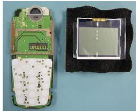
Place foil over display module for protection.
