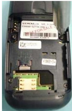
Remove the 4 screws (as indicated) with T5 Plus screw driver.
