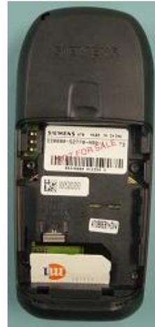
Remove SIM Card: 1) move latch upwards; 2) SIM Card will eject from holder
