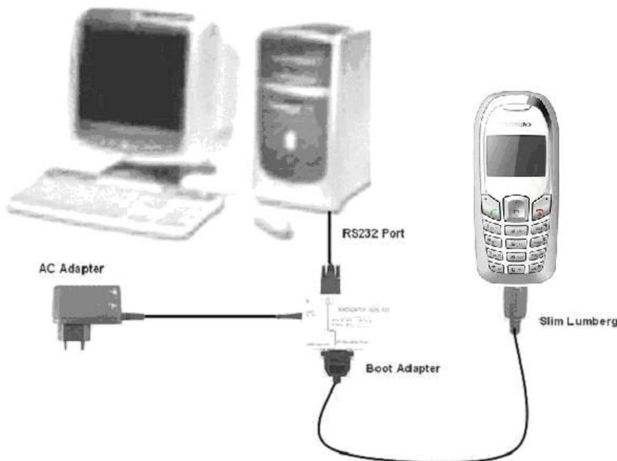
Figure 1. A70 Software Programming Setup
