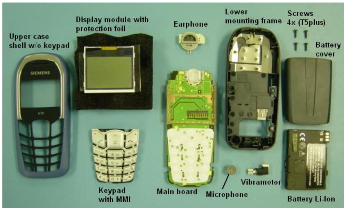
Fully disassembled A70
