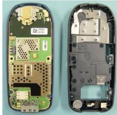
Remove Lower mounting frame with Vibra and Micro.
