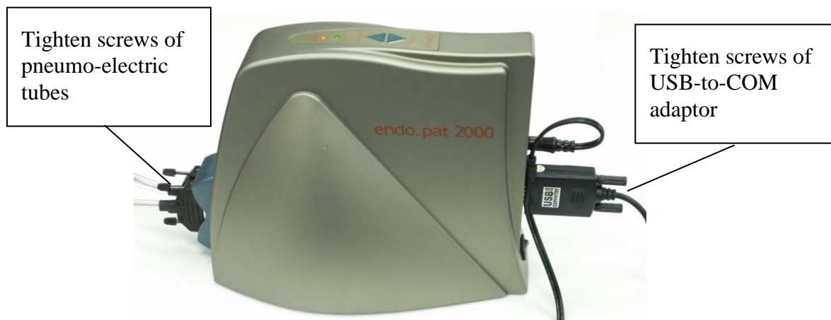
Figure 3 - Connection of pneumo-electric tubing and USB adaptor
