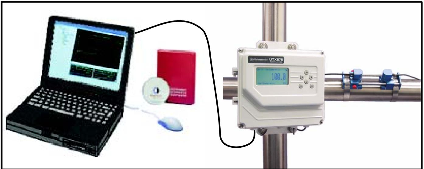
Figure 37: Connecting the UTX878 to a Computer Equipped with PanaView Software
