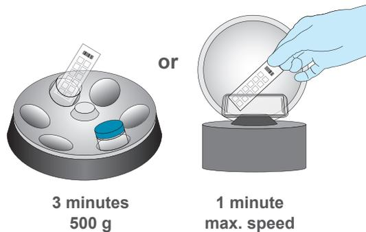
Figure 6: Working steps of the washing and drying procedure prior to the analysis of the CarnoCheck® chip with the CheckScanner™ and the CheckReport™ Software.
