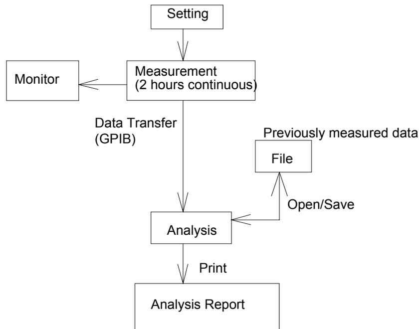
This program measures flickers generated from a device to be tested using a flicker meter that complies with IEC-868 and IEC-868-0 standards and calculates short period flicker values (**Pst**) and a long period flicker value (**Plt**). How much obstacle or flicker of lights is to be affected can be numericalized.
