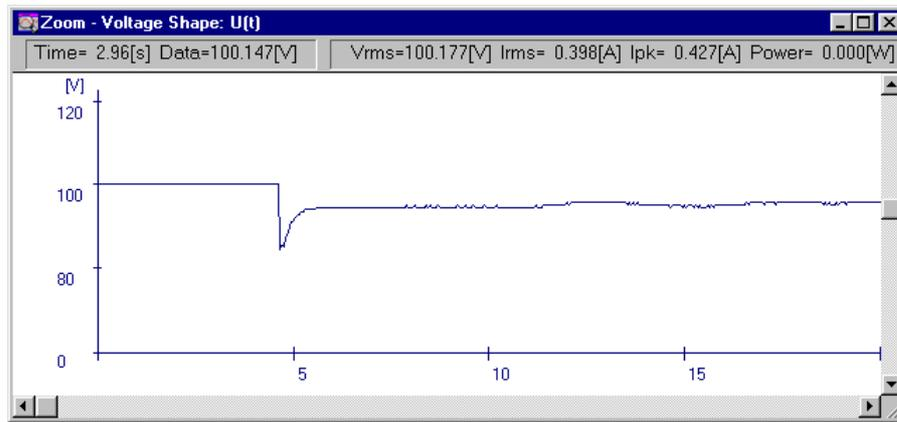
Data in a zoomed window will be represented on the ribbon (grey area aligned at the top of the window) instead of status line. The contents of data are exactly the same as that of base window. Although zoomed window cannot display entire data of 150 seconds at a time since its x-axis is expanded beyond VGA screen width, operating the horizontal scroll bar allows you to view entire scope.
