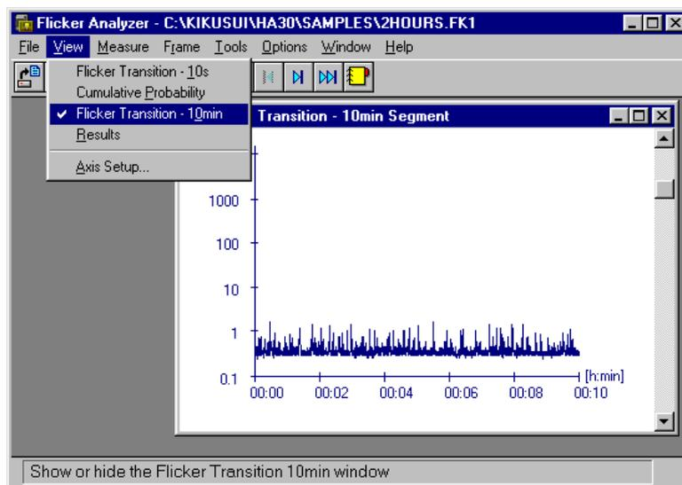
This window represents transition of PF values in a segment. The X axis indicates time elapsed from the beginning of the measurement, and the Y axis indicates the PF values. However, the X axis (time axis) doesn't display second unit portion.
