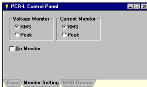
This page enables or disables voltage and current-monitor functionality. If you want to do it, check the **Do Monitor** check box. After returning to the **Panel** page, the monitor functionality will start.
