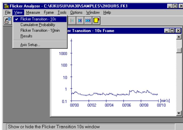
This window represents transition of PF values in a frame. The X axis indicates time elapsed from the beginning of the measurement, and the Y axis indicates the PF values. However, the X axis (time axis) displays only minute and second units but hour units. Be careful when you read the X axis if you do measurement more than one hour.
