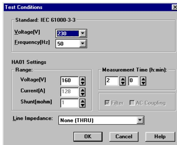
Select the **Measure | Test Conditions** menu. Then the **Test Conditions** dialogue will be shown. Items in the test conditions are roughly divided into two parts as described in subsequent sections.
