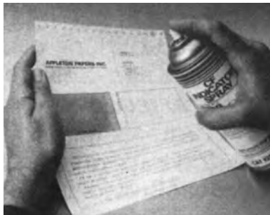
Checking CF Ink with CF Indicator Spray
