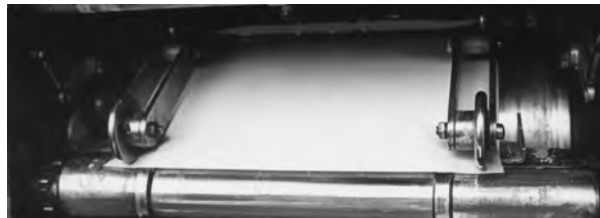
Setting ejector rolls outside of the ejector rings offsets upward curl in stock and sheet delivery will improve. See comparison.
