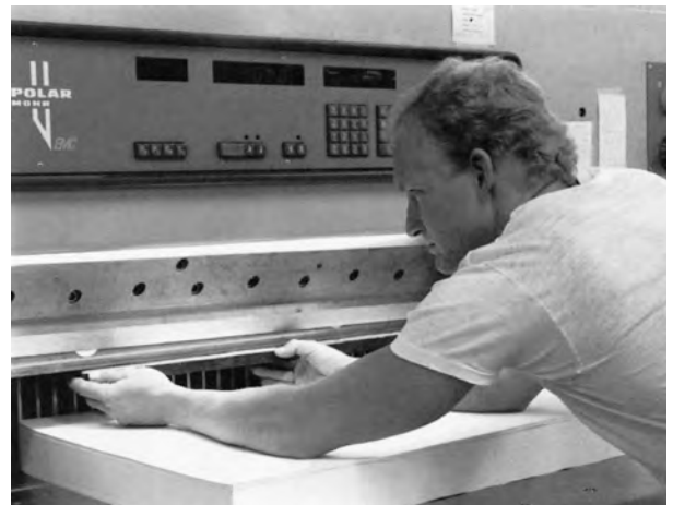
Sponge rubber pad is attached to bottom of the clamp bar. Chipboard stack prevents clamp damage to lift of paper. Proper trimming methods provide best results.
