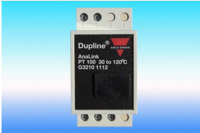
Photograph 14. Temperature transmitter type G3210 1112
