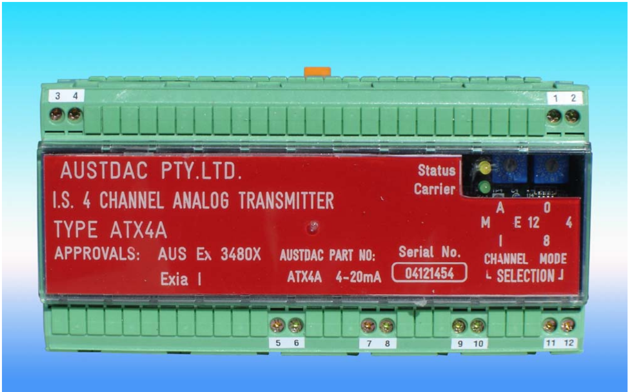
Photograph 11. Analogue transmitter type ATX4A
