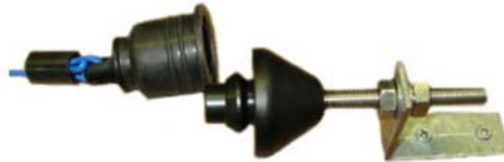
Photograph 27. Separated trip wire couplings used with the BMOS1
