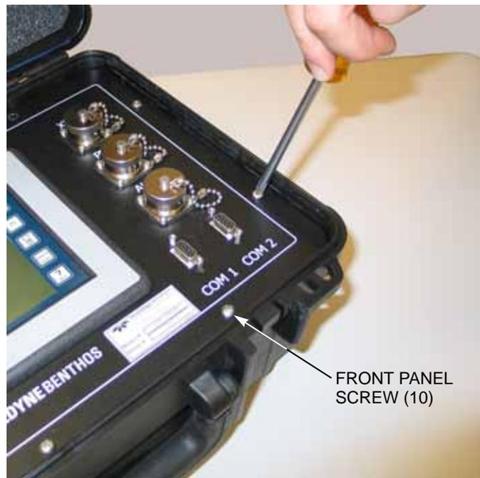
**Figure 6-1 Removing the Front Panel Screws**
