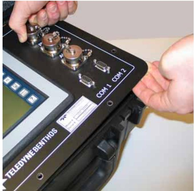
**Figure 6-2 Lifting the Edge of the Front Panel**
