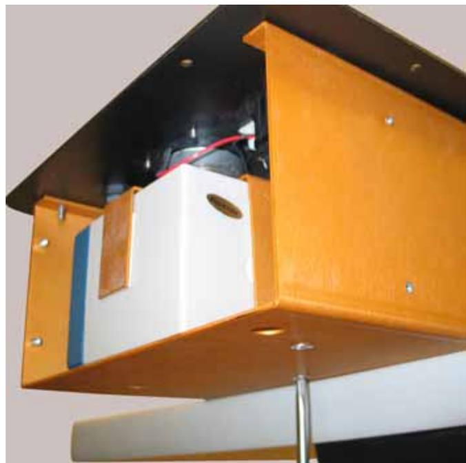
**Figure 6-5 Removing the Battery Bracket Screws**
