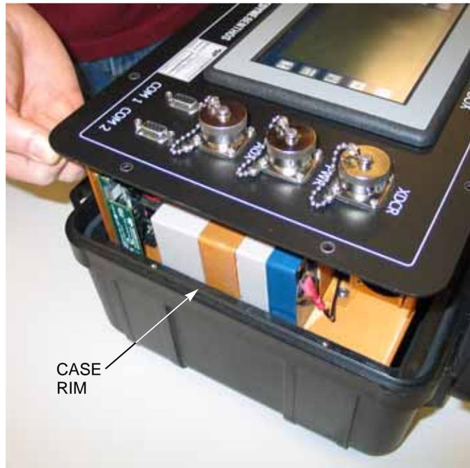
**Figure 6-8 Lowering the Electronics Chassis into the Case**
